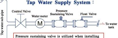
Pressure sustaining valve is utilized when installing pipes for users. It primarily matches up with the minimum working pressure inside the tap water pipe, balancing up-stream and down-stream pressure during normalcy and emergency, and maintains constant pressure inside the pipe.
